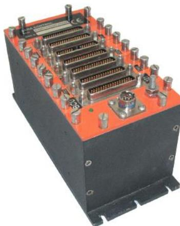
**Figure 2** Illustration of OTS Signal Data Converter
